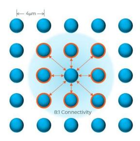
With Atom Computing's system, site-specific single-qubit gates can be executed in parallel in rows across the array, which increases the overall efficiency of the system. Two-qubit gates can be performed between qubits and their nearest neighbors.
